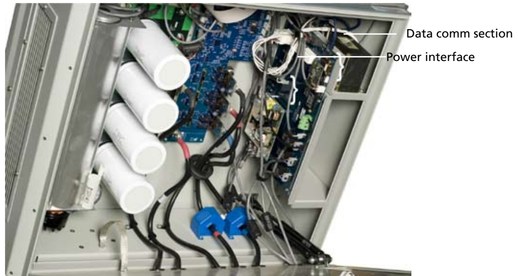
Figure 5-1 Power interface and data comm sections on PVP30kW inverter
